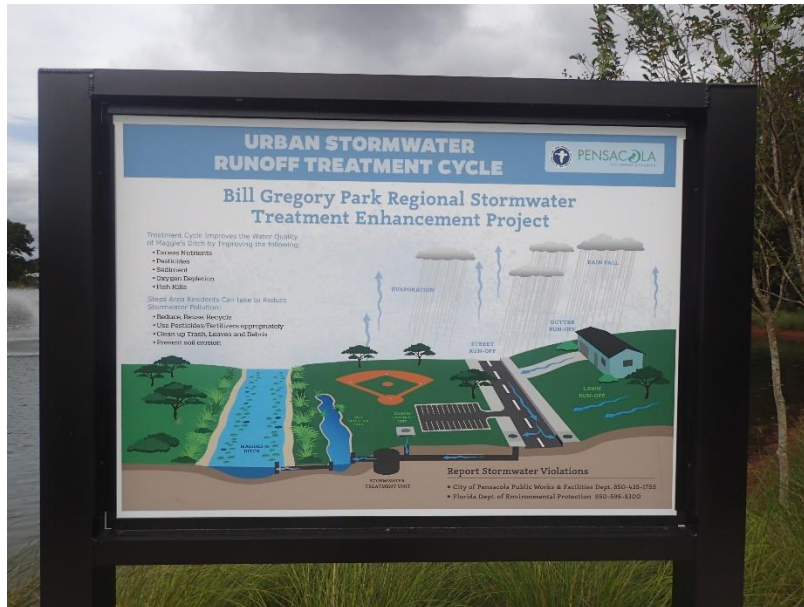
Photo 2. The new stormwater pond at the Bill Gregory Park (Bayou Chico Watershed) at W Street was funded by a NFWF grant for the City of Pensacola with pass thru assistance by EsCo. This stormwater pond was designed to treat 38 acres of stormwater before entering the Maggie’s Ditch, a small tributary.
