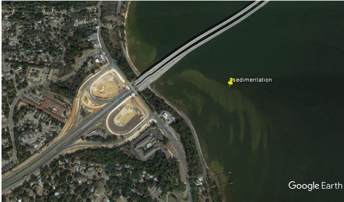
Aerial view of I-10 and Scenic Highway in Escambia County, FL, adjacent to Pensacola Bay. Note the sedimentation in the bay and the large stormwater ponds roughly 4 acres in size each – the median is still visible in this view from Google Maps, February 2015.
